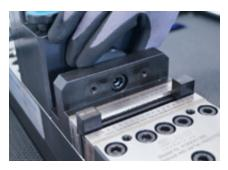
Position one gauging block with slots on each side of the stamping jaws. Tighten the jaws by hand only, do not actuate the switch!
