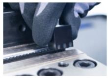
Make sure that the stamping teeth are placed in the grooves of the gauging blocks.
