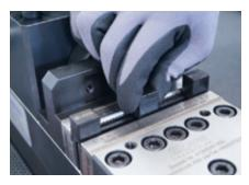
When the indicator block fits between the stamping contour, the jaws need to be sent in for reconditioning.
