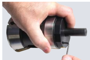
Lock stopper housing in position
