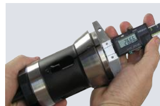
Adjust stopper shaft position
