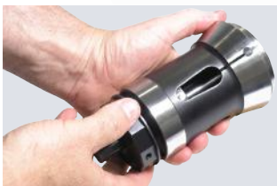
Insert collet work stopper
