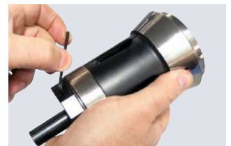
Lock stopper shaft and install
