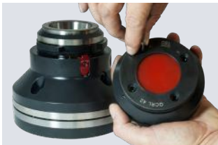
Remove bar seal from housing
