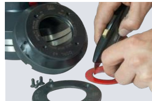
Cut out the diameter
