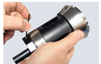
Lock stopper shaft and install
