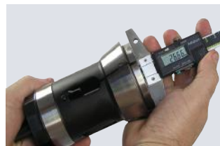
Adjust stopper shaft position
