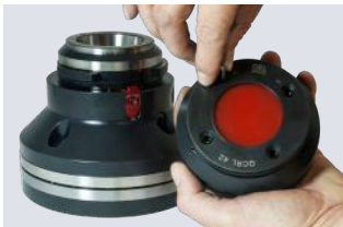
Remove bar seal from housing
