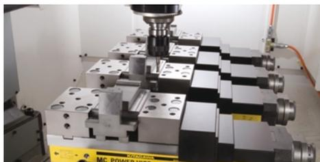
▲The standard parallel specification enables simultaneous machining of multiple workpieces, thus reducing costs.
